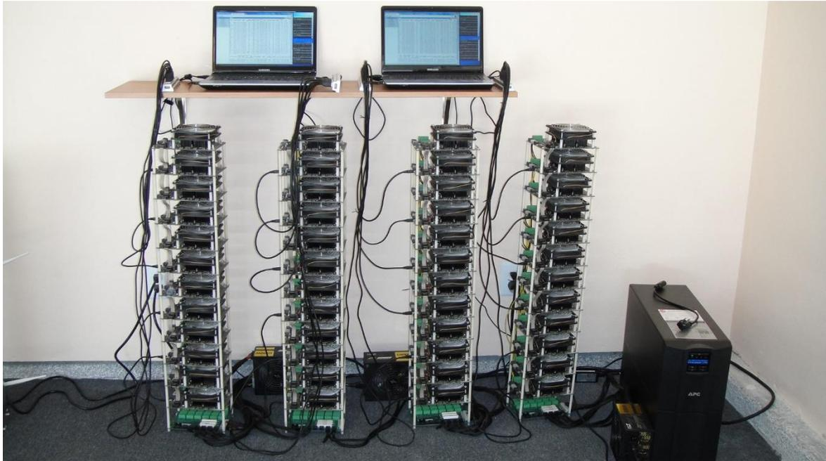
The first FPGAs were initially announced on the bitcointalk forums and offered 100-400 MH/s. At the time FPGAs were first introduced, the cost/benefit was questionable with top-end GPUs able to run at 700 MH/s, but they did offer additional benefits. Notably, a single computer could run stacks of FPGA miners, compared with just a few GPUs under normal conditions.
